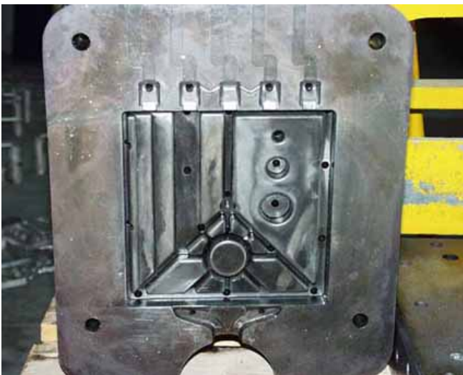
Figure 4. The die used for gating system optimization
