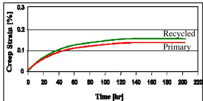
Figure.5. Creep strain achieved in MRI 230D alloy for 200 h testing at 180°C under stress of 70 MPa
