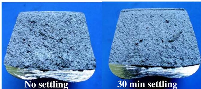
Figure 4: Visual appearance of MRI 230D coupon fracture surface after settling at 690°C of 30minuts. (No bubbling was performed)
