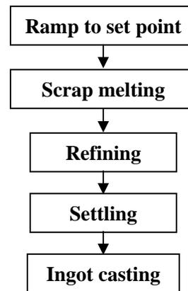
Figure 1. Flow chart of the recycling process
