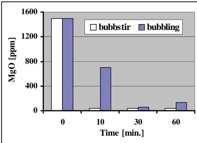
Figure 3. Reduction of the MgO content in MRI 230D melt depending upon settling time at 690 °C and type of recycling procedure.
